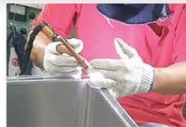
Butt Welding: the joints on the sink rim are butt welded.
