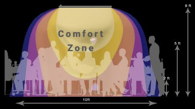
Example: For an ambient temperature of 35 °F and wind conditions "Still Air", one long wave heater with 3200 W input mounted 8 feet above the floor provides a comfort zone coverage area of 10ft x 8ft.
