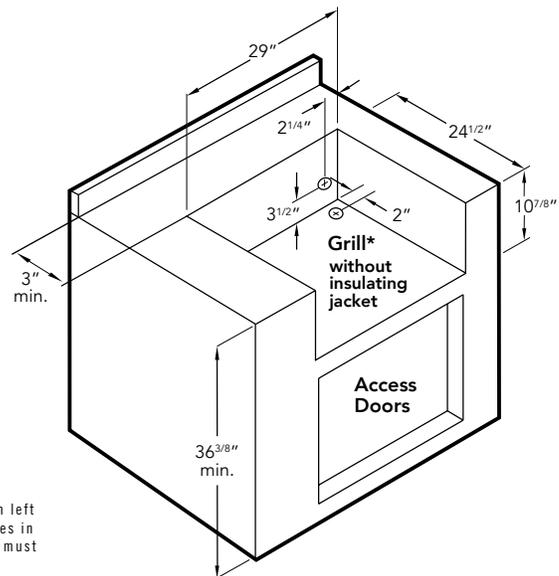
4" square holes for gas and electrical connections both left and right sides (rear or bottom access). Make these holes in the frame based on your requirements. 120V GFI outlet must be located within 6" of the 4" hole.
