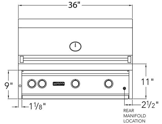
4" square holes for gas and electrical connections both left and right sides(rear or bottom access). Make these holes in the frame based on your requirements. 120V GFI outlet must be located within 6' of the 4" hole.
