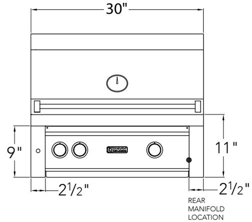
4" square holes for gas and electrical connections both left and right sides(rear or bottom access). Make these holes in the frame based on your requirements. 120V GFI outlet must be located within 6' of the 4" hole.
