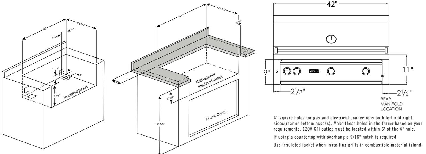
4" square holes for gas and electrical connections both left and right sides(rear or bottom access). Make these holes in the frame based on your requirements. 120V GFI outlet must be located within 6' of the 4" hole.
