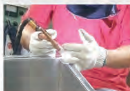
Butt Welding: the joints on the sink rim are butt welded.
